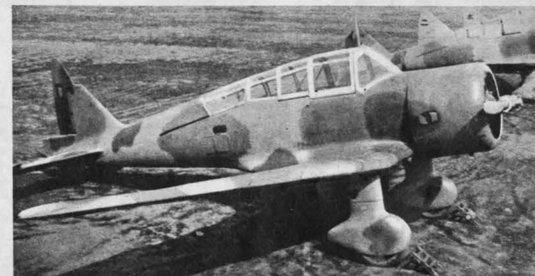
Ida is an old reconnaissance plane, now used as an army trainer. The thick fuselage and faired cabin make Ida appear exceptionally small, but its span and length approximate those of Babs.
